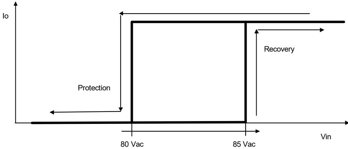
● **Input Over Voltage Protection Diagram**
